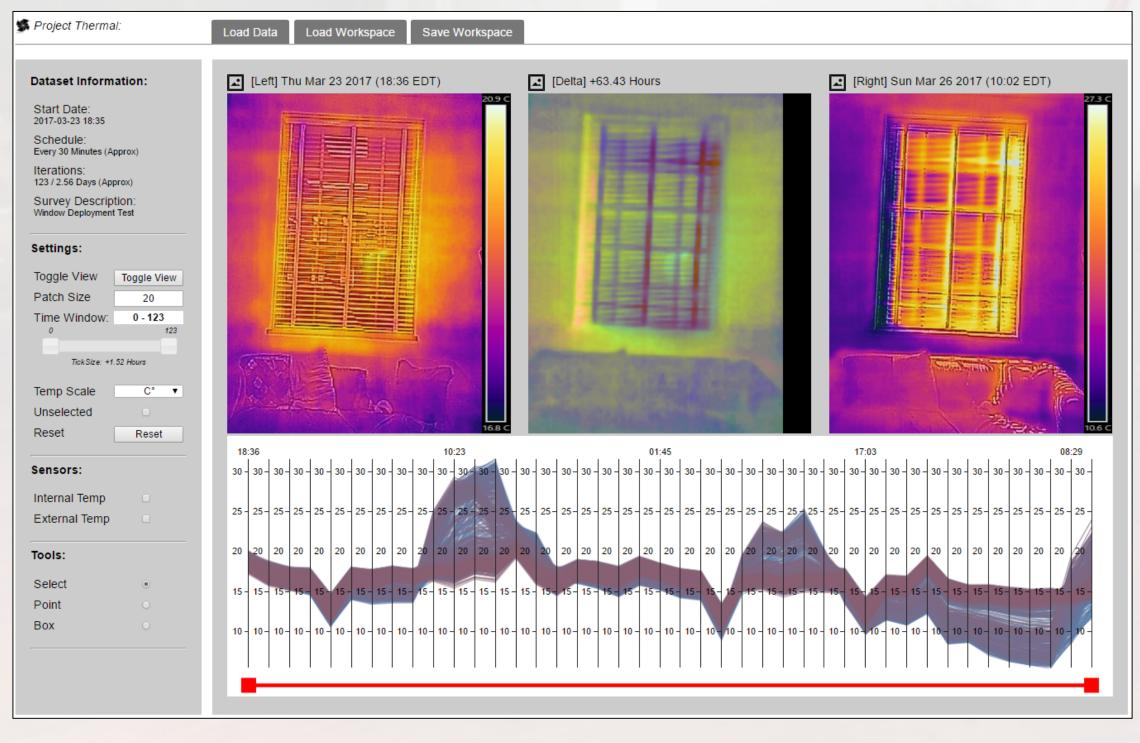
Our temporal analysis tool is centered around a Parallel Coordinate Plot of the temperature changes between the collected images; this plot visualizes the trend of the temperatures at each pixel location as images are spatially aligned. We also overlay sensor data on this plot and allow the user to scan through the images to make point-in-time comparisons and derive insights.
