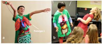
**Figure 1:** *BodyVis* is an interactive e-textile shirt for body learning that actively responds to the wearer's physiology and visualizes their body data on externalized anatomical models. Prototypes 1 and 3 shown above.
